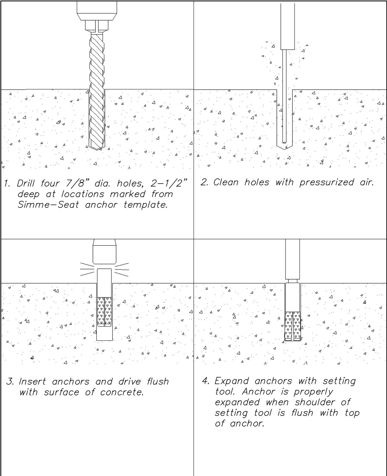
1. Drill four 7/8" dia. holes, 2-1/2" deep at locations marked from Simme-Seat anchor template.
